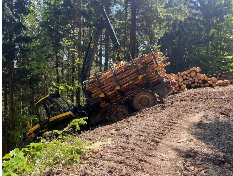
Figure 15: Cable assisted forwarder © Klara Voggeneder
